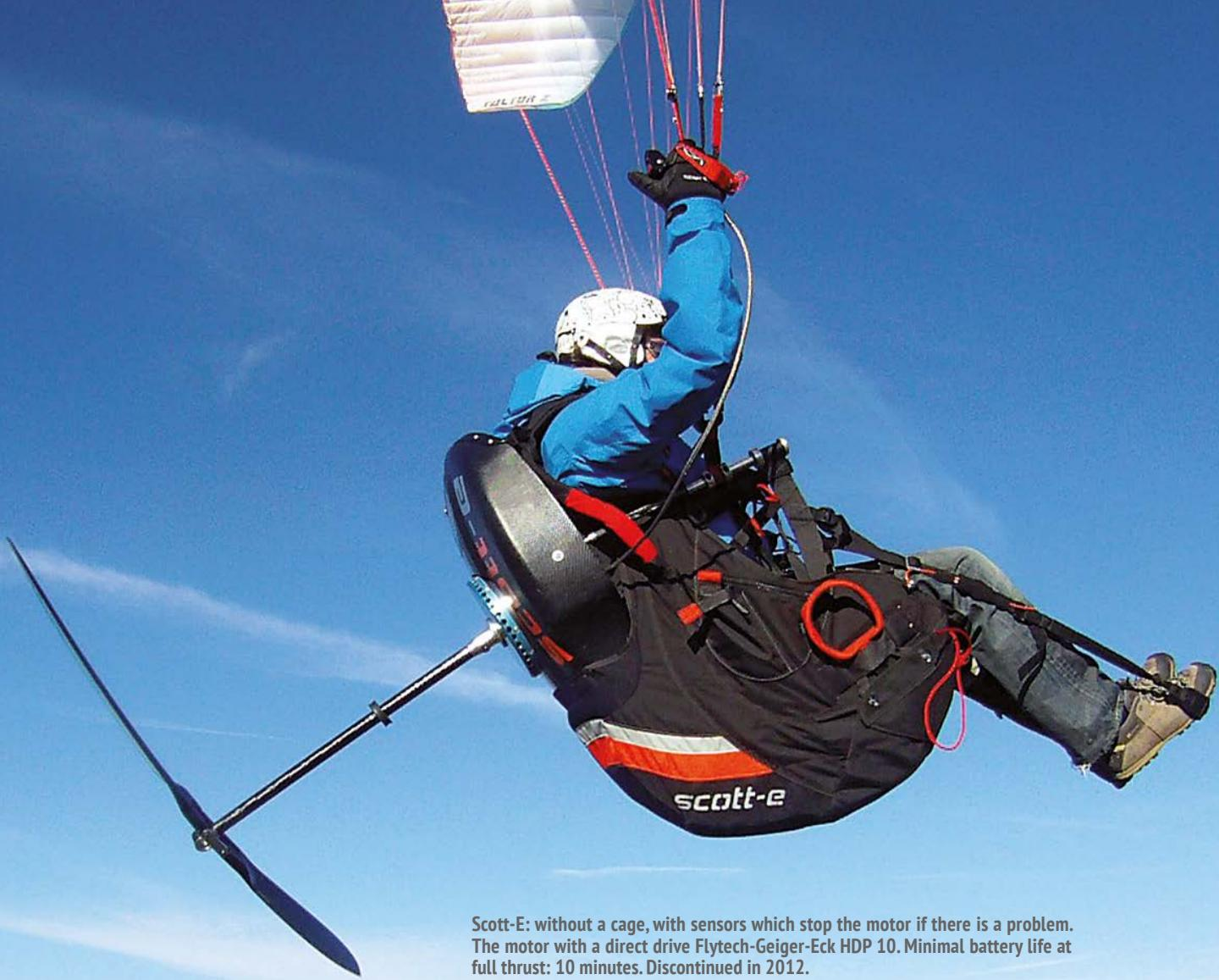
Scott-E: without a cage, with sensors which stop the motor if there is a problem. The motor with a direct drive Flytech-Geiger-Eck HDP 10. Minimal battery life at full thrust: 10 minutes. Discontinued in 2012.
