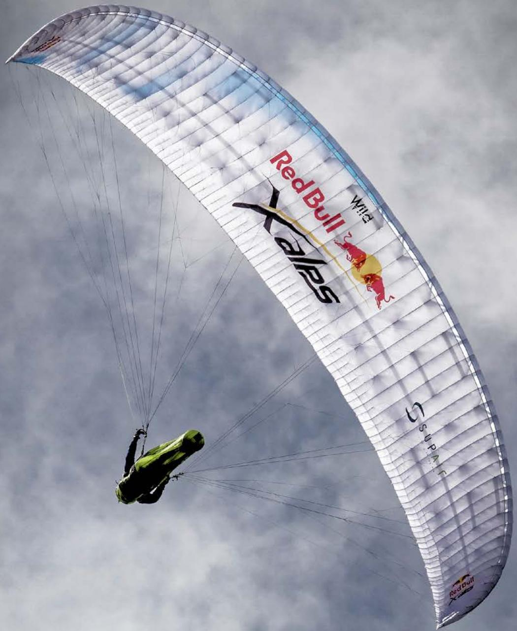
Benoit Outters on his Wild, which clearly reveals its internal structure in this beautiful photo by Nolas Assel. It's a three liner, derived from the Supair Taska, with a higher aspect ratio and an EN D instead of an EN C.
