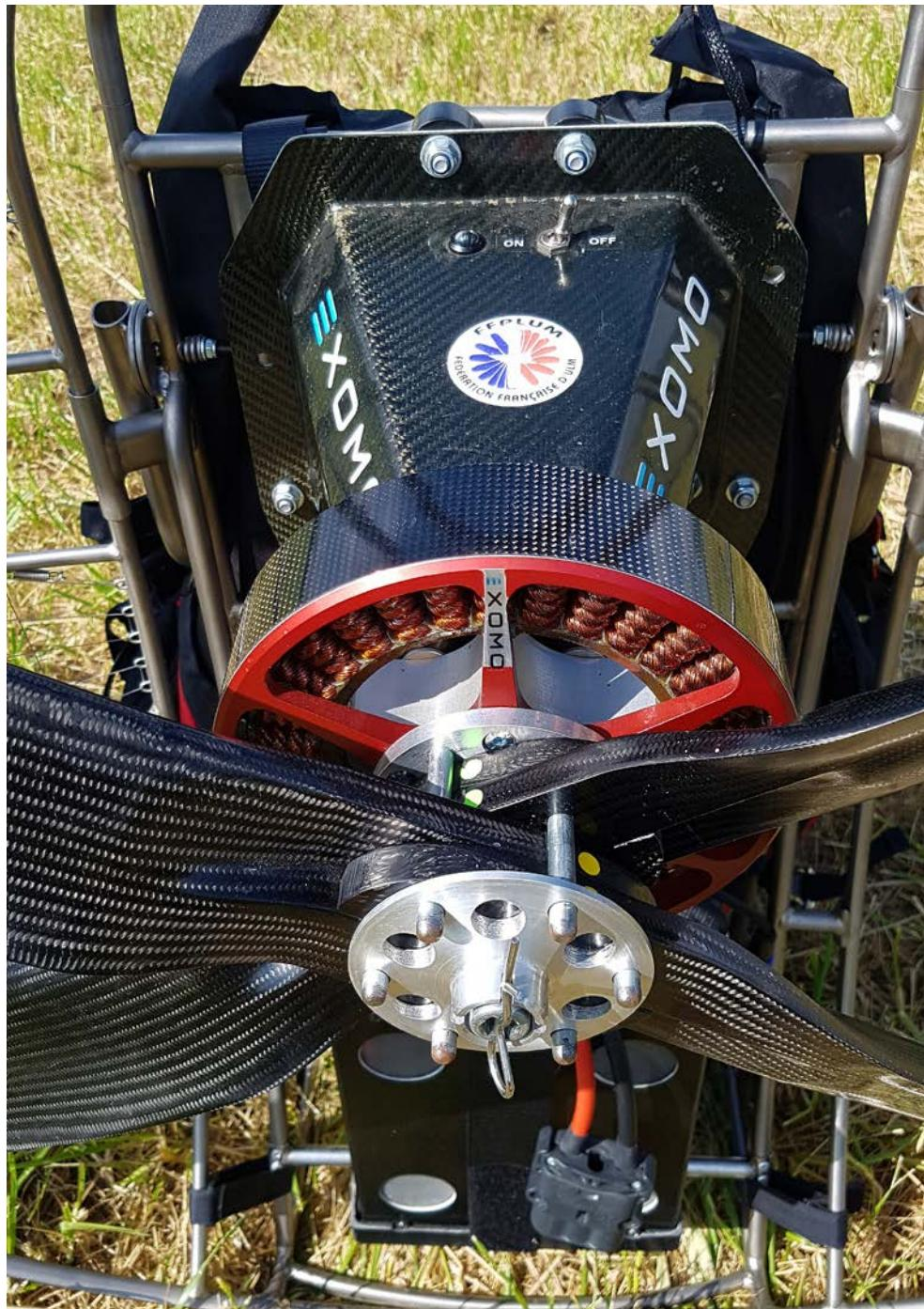
Pre-flight checks are reduced to a minimum given that the 'heart' of the electric motor is protected by a carbon case. Master switch to ON, a push of the thumb on the control button, a three second wait, a beep ... and then you're off!
