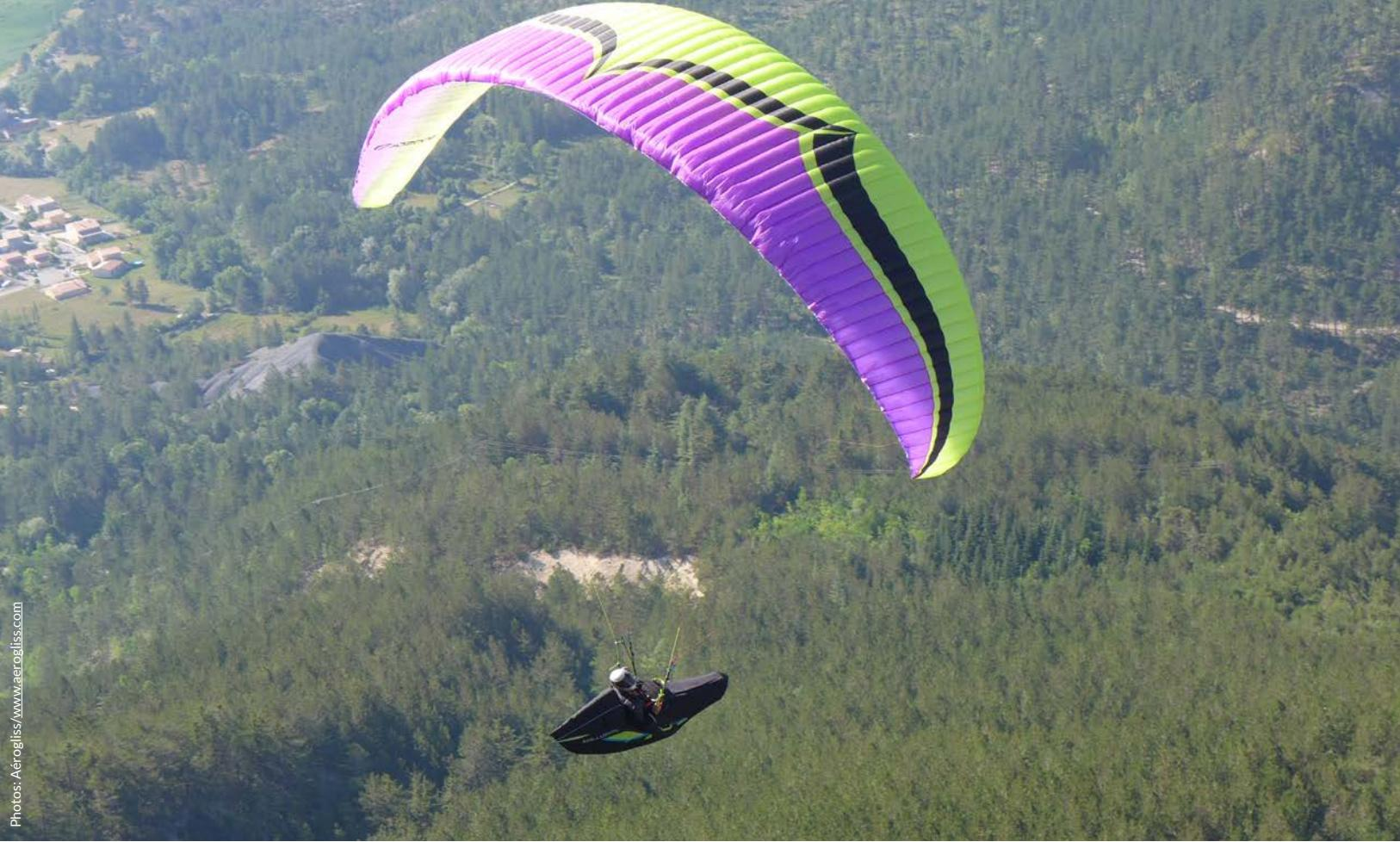
The wing breaking between the Bs and Cs and emptying of air, that was sometimes seen briefly in the second version, has totally disappeared. Therefore it's a straightforward, well behaved wing!
