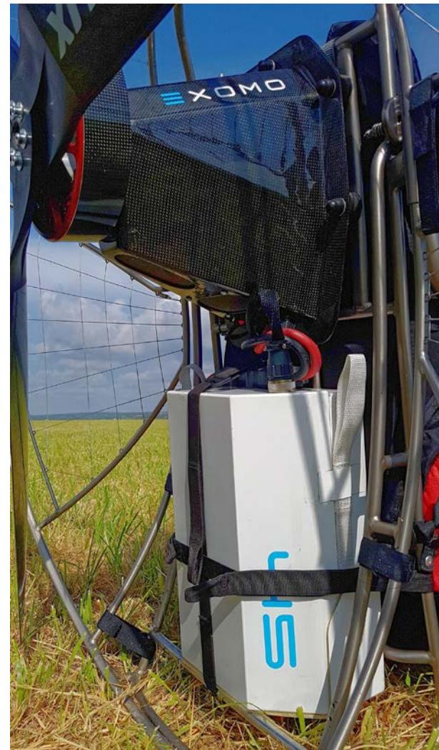
The motor is protected by a very smooth carbon cover.
