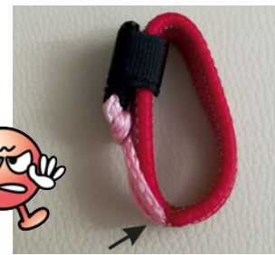
The connector is made with a single thread in the middle. Above all, once put together, the weak part will be in a place which is heavily used.
